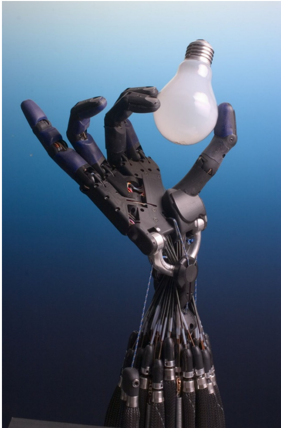
Fig: 6 From this picture threads and nylon can be used for moving fingers.
